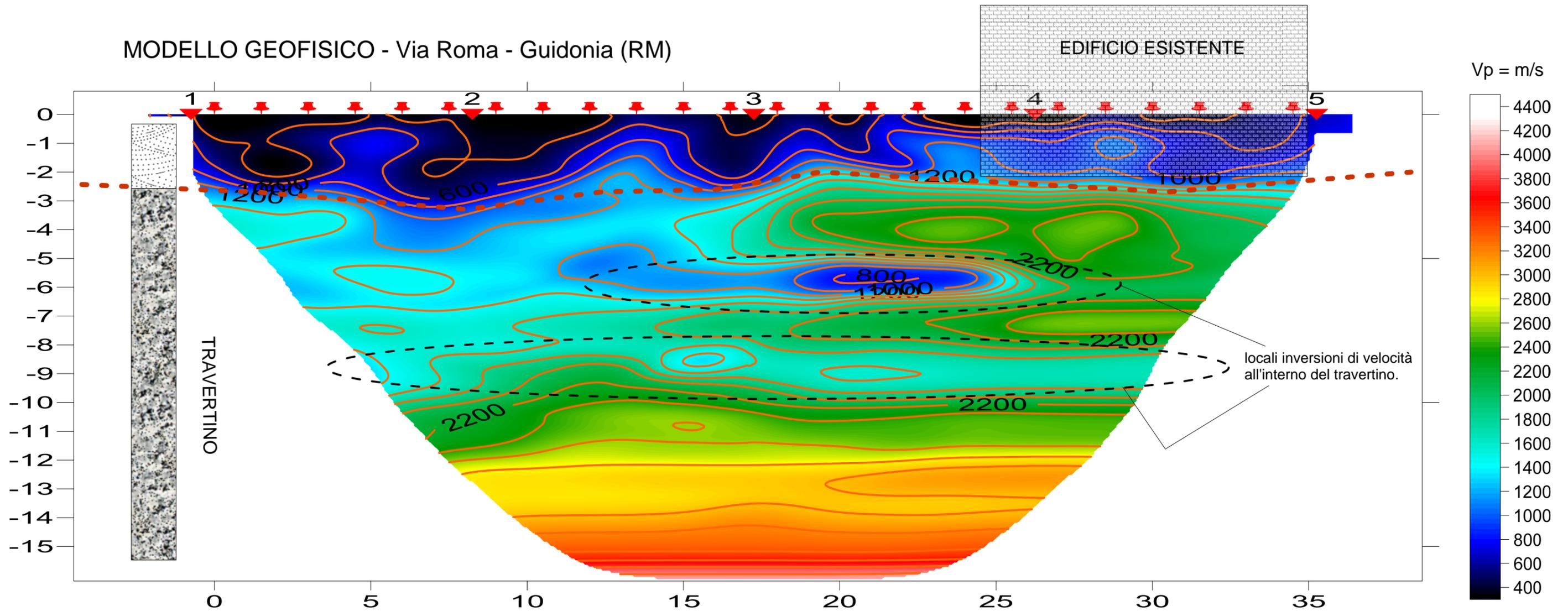
FIORITO, 10 WET iterations, RMS error 7.3 %, 1D-Gradient smooth initial model, Version 3.17
